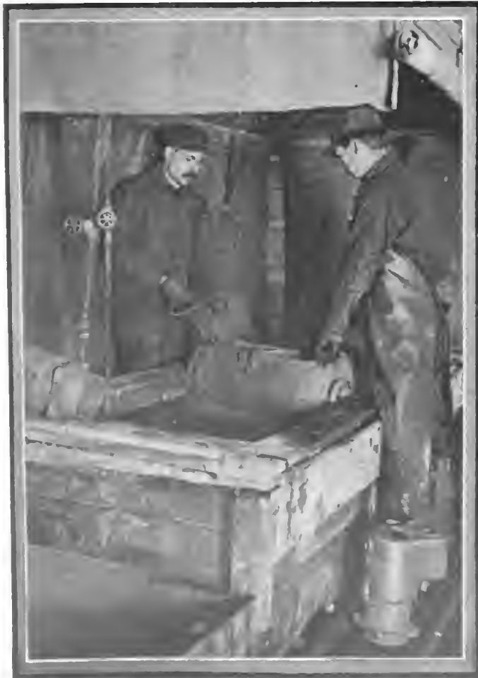
Fig. 2—Workmen dipping cylinder and other castings in pickling vat, previous to machining operations.
